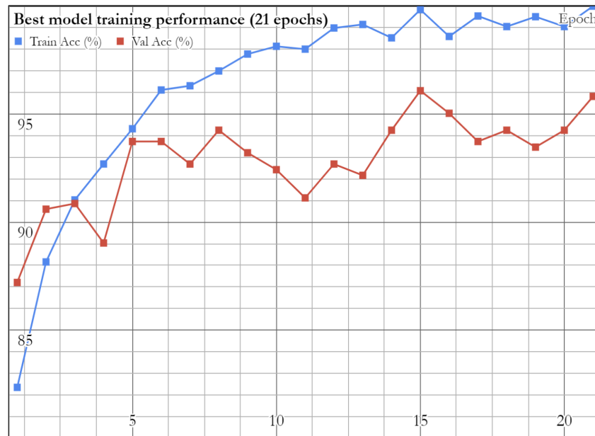
Figure 7: The training and validation accuracy of our best model over 21 epochs. The best performing model was reached after 15 epochs
